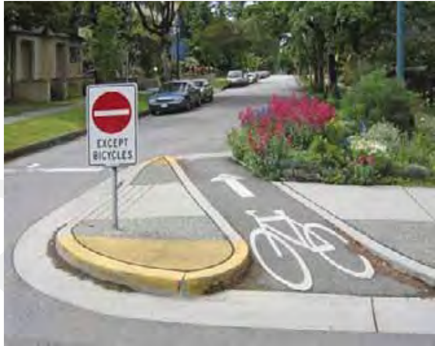
Figure 1. (Partial motor vehicle diverter: Bicycle-only entrance, all vehicles may exit.)
