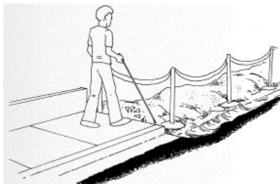
Figure 10-5. PROBLEM: Construction sites should include temporary ramps and should be blocked off with solid fencing. The thin tape in this illustration is not detectable using a long white cane.
